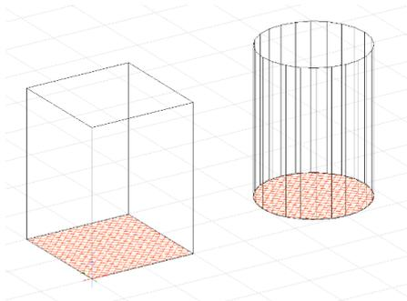
*Polyslab and cylinder 2D contour (red) with height*
