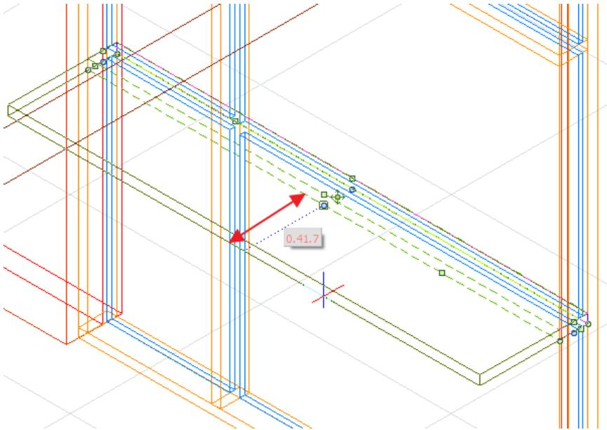
*Polyslab move edge - vertical dimension input*
